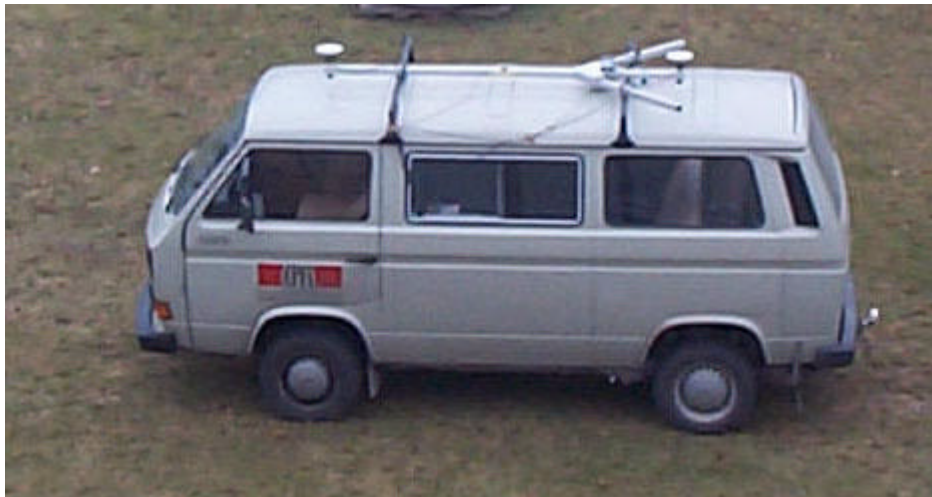
Figure 3 A view of the high precision measurement vehicle equipped with several GPS receivers and a dead reckoning system
